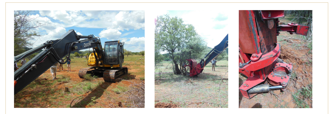
Figure 5.2 - Tambuti Wilderness Farm: the extendable arm on the caterpillar and the scissor appliance
