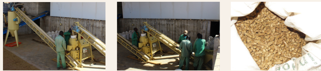
Figure 5.9 - Pelletizing line at Langbeen Farm with a sample of the pellets (the size of the pellets is 8 mm)
