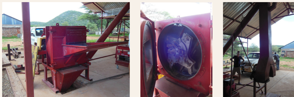
Figure 5.10 - Hammermill at BosPro Products connected to a bag-filling machine that facilitates production and packaging
