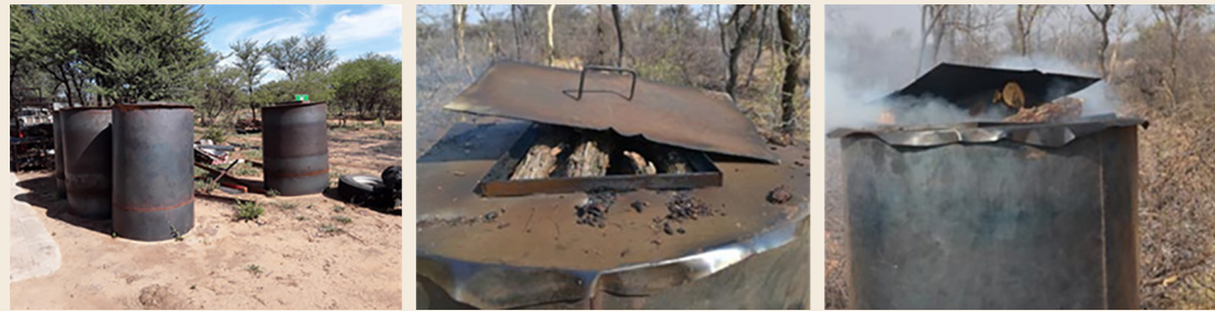
Figure 8.6 - Drum kilns built in Otjiwarongo and working for Otjiwarongo (Makarra bush products)
