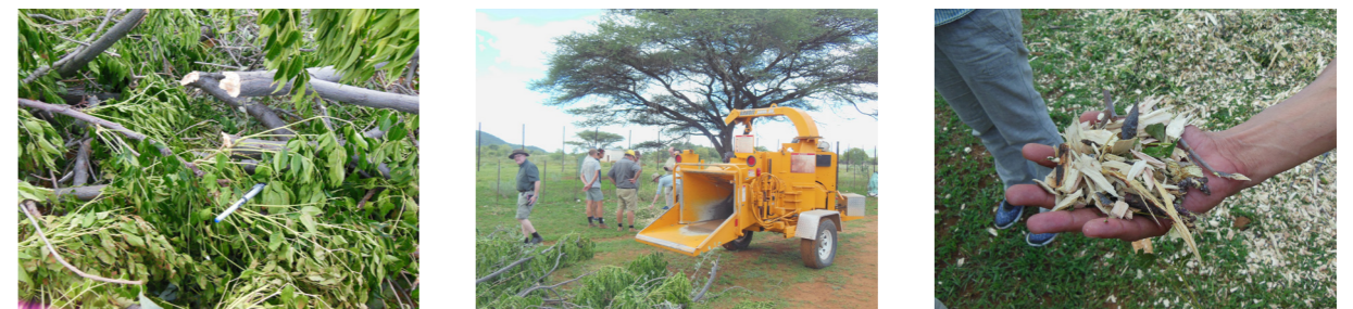
Figure 5.7 - Images showing the harvested bush material, chipping machine, and chips produced at BosPro Products
