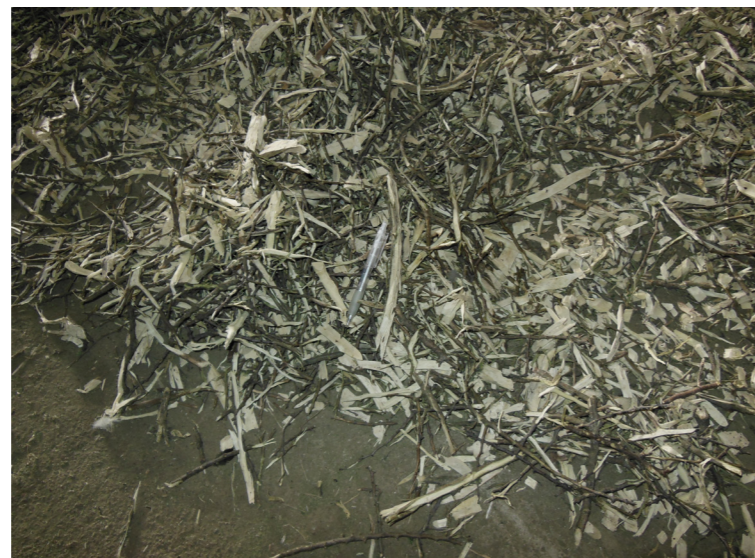
Figure 5.5 - Junkkari HJ 250 GT chipper, imported from Finland and in use at UNAM, Neudamm Campus (20 km east of Windhoek) and wood chips measuring an average 3 cm x 7 cm in size
