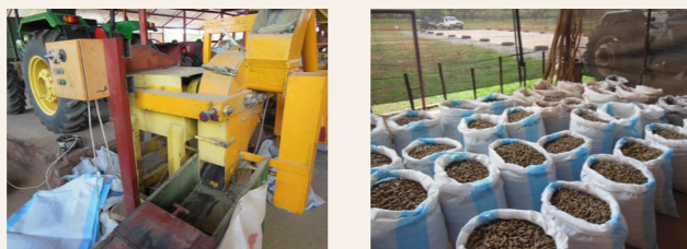
Figure 5.13 - Pelletizing machine at BosPro Products and, 50-kg size bags filled with freshly made pellets
