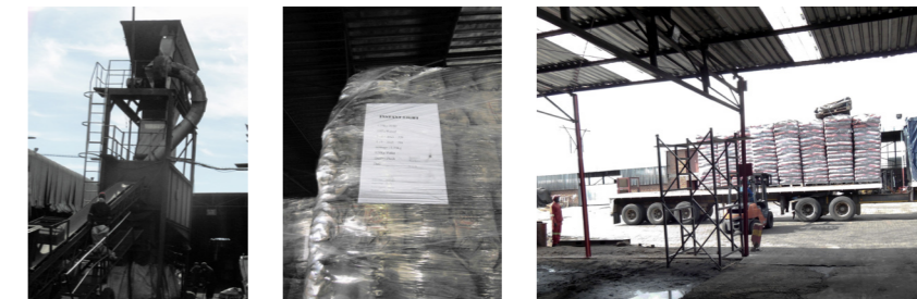
Figure 5.16 - Jumbo Charcoal’s operation 4 km west of Okahandja: the sifter uses gravity to drop the charcoal down where it is separated according to size
