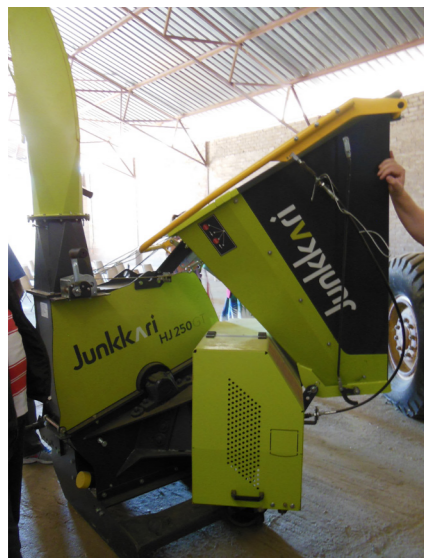
Figure 5.5 - Junkkari HJ 250 GT chipper, imported from Finland and in use at UNAM, Neudamm Campus (20 km east of Windhoek) and wood chips measuring an average 3 cm x 7 cm in size
