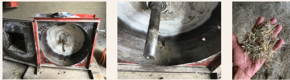
Figure 5.8 - Damaged Drotsky Hammermill at Neudamm Agricultural Campus
