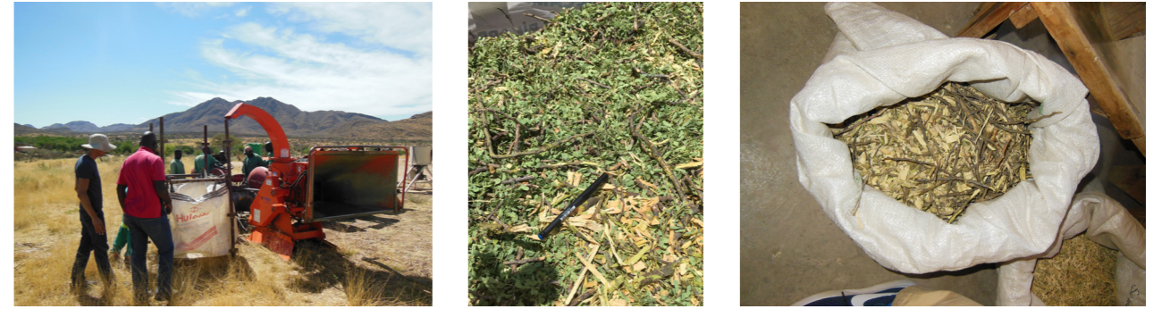
Figure 5.6 - Images showing the chipping machines and chips produced at Langbeen Farm, Dordabis, northeast of Windhoek
